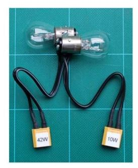
In practice this is a cheap and simple configuration that safely covers discharge requirements for the most common packs.
